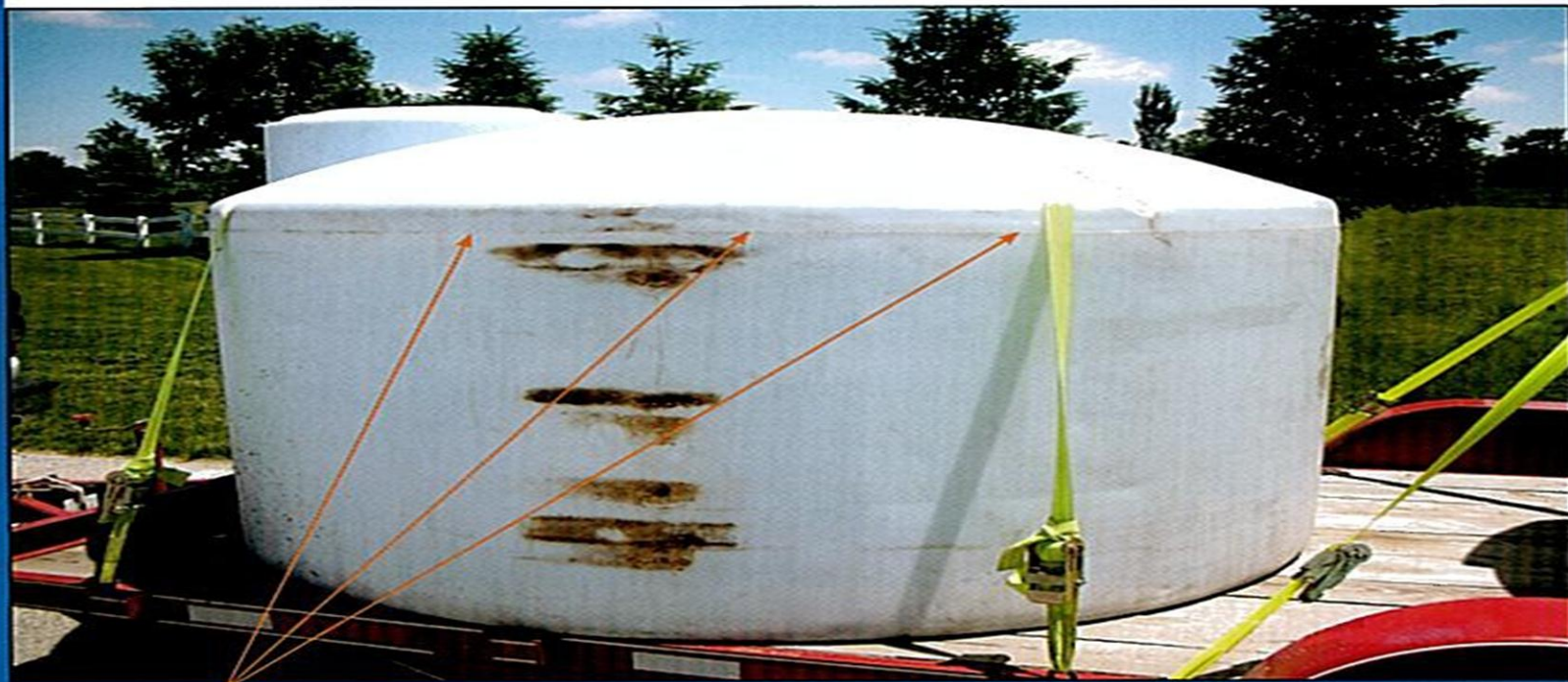
Notice the parting line on this tank.
